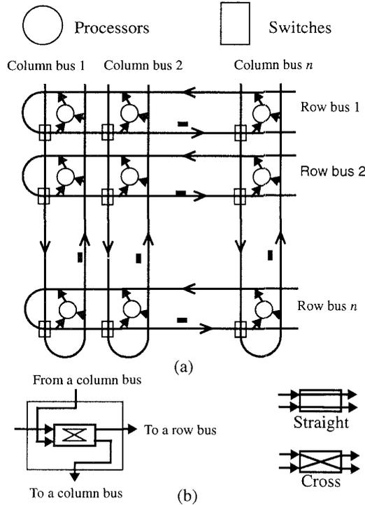
**Figure 1.** (a) The architecture of RASOB, and (b) A switch interconnecting a row and a column bus.
