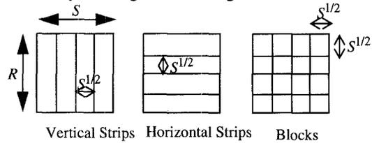
**Figure 4.** Partitions of the  $R \times S$  array.
